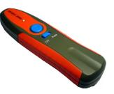
The universal connector can be used for all the most widespread fiber interfaces such as ST / SC / FC connector. It is suitable to test both Singlemode and Multimode cables. With an optional 2.5 mm to 1.25 mm optional Adapter, you can easily test 1.25 mm diameter fiber LC or MU connector. The visibility is from 3 km to 5 km dependent upon the output power of the Fiber Checker.
