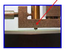
krell technologies www.krelltech.com Tech Support: 732-617-7091 **Step 2:** Pull pin, and raise the pressure applicator bar to the uppermost position. Bottom-out the fiber adapter in the workholder fixture. Orient with the registration mark facing forward. Lightly lock into position.
