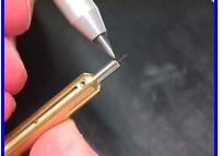
As an option, insert fiber into adapter, and score with a scribe tool just beyond the ferrule tip
