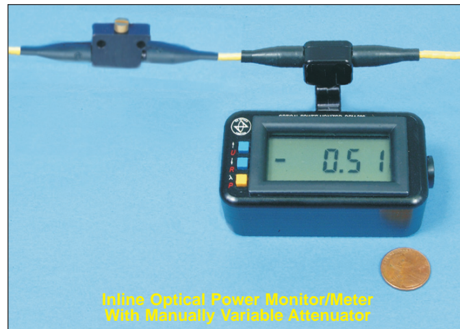
Inline Optical Power Monitor/ Meter With Digital Display
