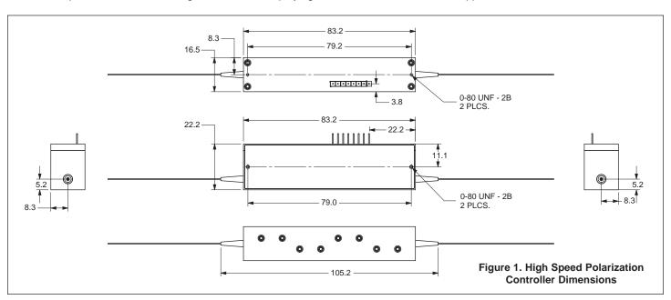
The polarization controller is available in either a three or four channel configuration. The three channel system is ideal for polarization scrambling applications such as for polarization averaging, PDL or PDG measurements. The added redundancy of the four channel version opens the way to continuous polarization control, without having to occasionally reset the device when a controller reaches its limit.
